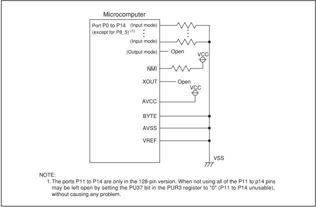
Figure 19.12 Unassigned Pins Handling
